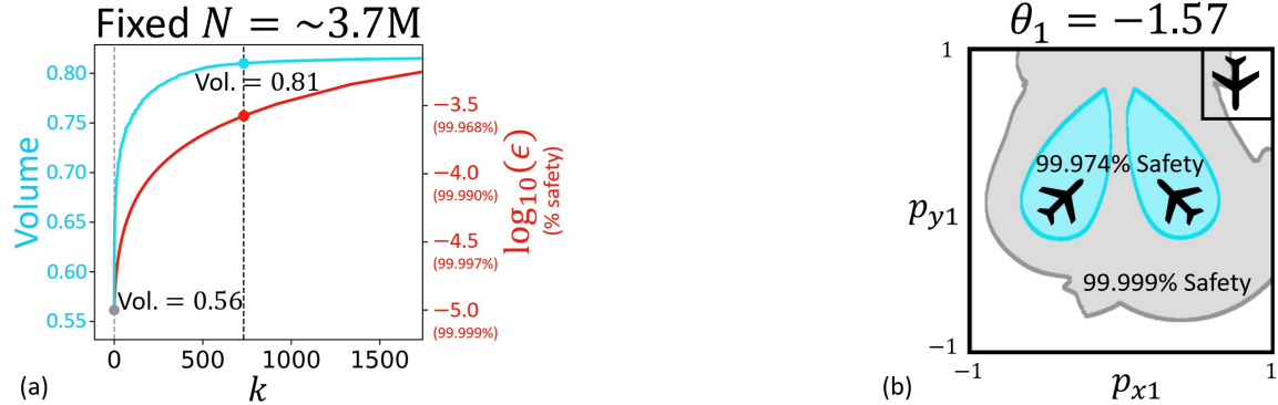
Figure 1: (Left) For a fixed simulation budget N , the cyan curve shows the number of empirical safety violations k for different learned volumes (different super-levels of \tilde{V}(x, 0) ). The red curve shows the trade-off in safety strength \epsilon (in log scale) for each k using the robust method. The grey point indicates the iterative method baseline. The robust method is able to provide safety assurances even for the volumes that have non-zero outliers. (Dashed black line) By a small decrease in safety level (from 99.999% to 99.974%) caused by outliers, we are able to significantly increase the assured safe volume from 0.56 to 0.81. (Right) The BRT, the complement of the safe set \mathcal{S} , shrinks greatly (from grey to blue).
